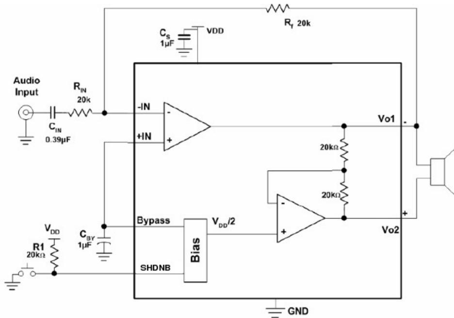
Figure1. Audio Amplifier with Single-ended Input
