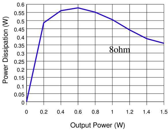
Power Dissipation vs Po, VDD=3V
